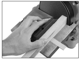
Figure 13. Mitering with the table angled.
